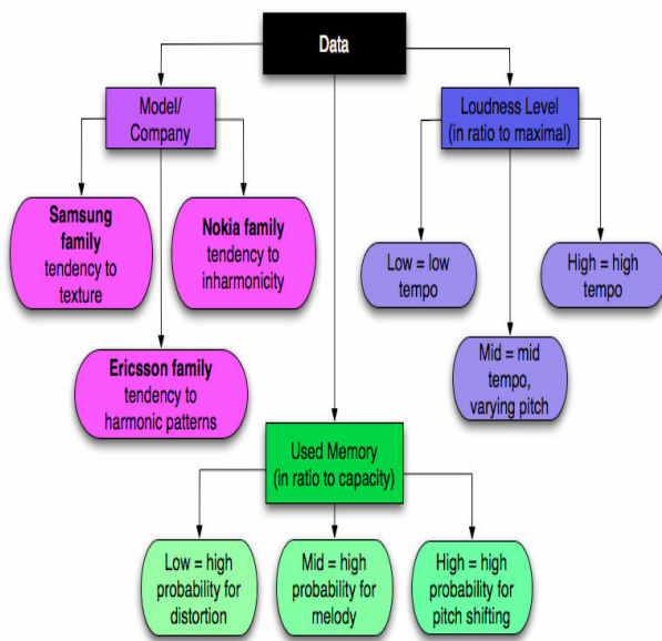
Figure 2.: Simplified example of data mapping to musical parameters in the audio engine. Data from the mobile device is classified in three groups – Model/Company, Loudness Level, Used Memory. These are being mapped to variables and control parameters in the audio engine, varying the characteristics of the sound and the structure of the composition.
